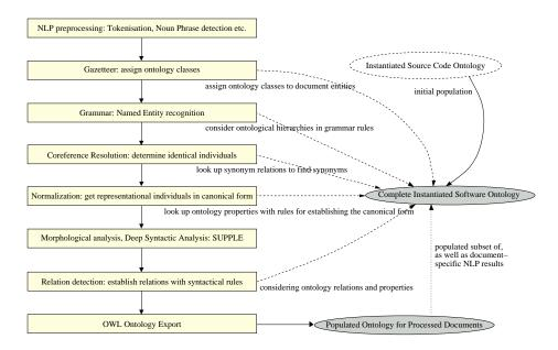
Fig. 3. Workflow of the software text mining subsystem
